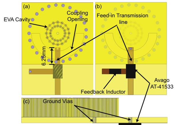
Fig. 5. Schematics of the proposed oscillator (Bias line is not shown) (a) front-view (b) back-view and (c) side-view.
