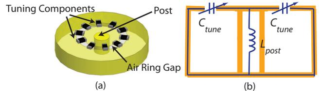
Fig. 1. Schematic of resonator design: (a) PCB with generalized varactor as tuning elements; (b) equivalent circuit model for the proposed air ring gap cavity [4].
