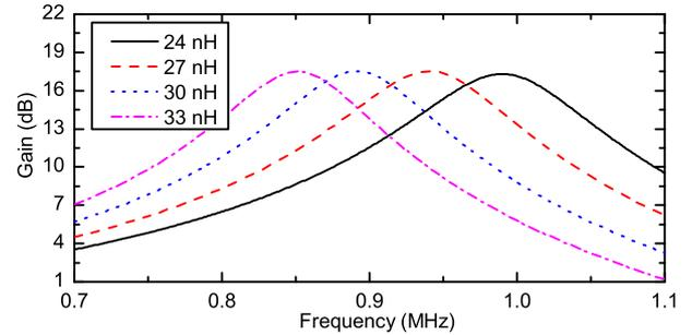
Fig. 4. Amplifier power gain under different feedback inductance.
