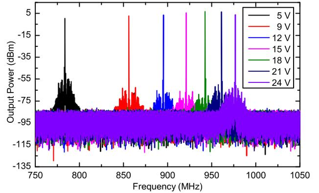
Fig. 8. Measured oscillator tuning range
