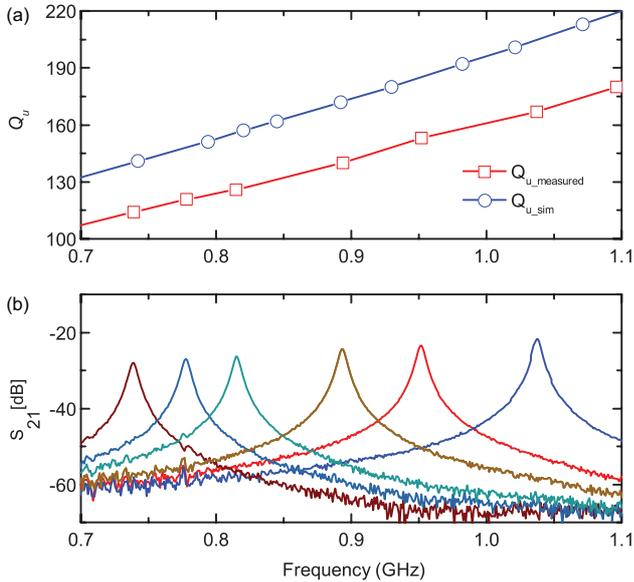
Fig. 2. (a) Simulated and measured  $Q_u$  over tuning frequency and (b) measured  $S_{21}$  of the resonator.
