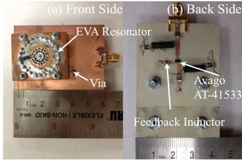
Fig. 6. (a) Front side of the oscillator and (b) back side of the oscillator.
