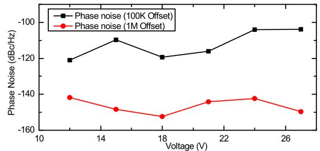
Fig. 9. Phase noise measurement over the tuning voltage
