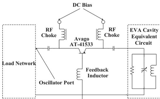
Fig. 3. Two port negative-resistance oscillator circuit topology.
