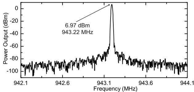
Fig. 7. Spectrum of oscillator output at bias voltage of 18 V.
