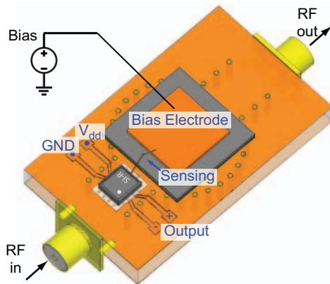
Fig. 8. Concept illustration of a MEMS tunable evanescent-mode cavity resonator with integrated monitoring circuitry.
