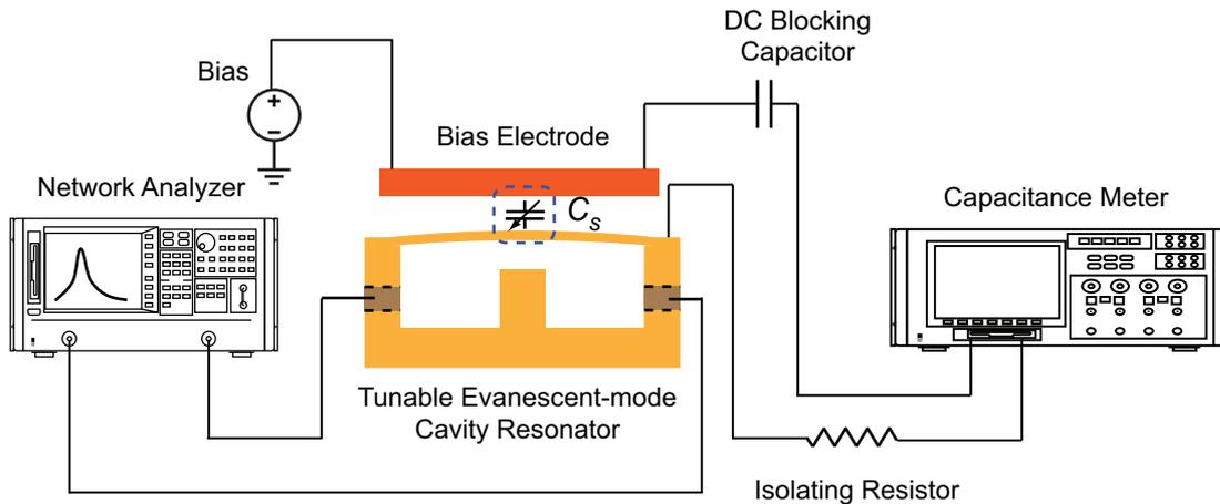
Fig. 5. Block diagram of the measurement setup.
