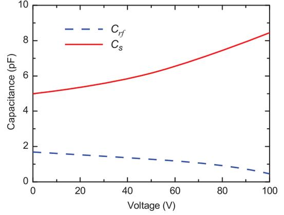
Fig. 3. Calculated  $C_s$  and  $C_{rf}$  with respect to bias voltage. The calculation assumes the following parameters: initial gap  $g_0 = 5 \mu\text{m}$ , electrode size  $6 \times 6 \text{ mm}^2$ , and actuation gap  $d_0 = 60 \mu\text{m}$ .
