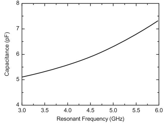
Fig. 4. Calculated  $C_s$  with respect to the resonant frequency using the same parameters are assumed in Fig. 3.
