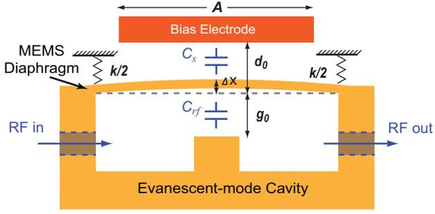
Fig. 2. Spring-mass model of the MEMS tunable evanescent-mode resonator [6].
