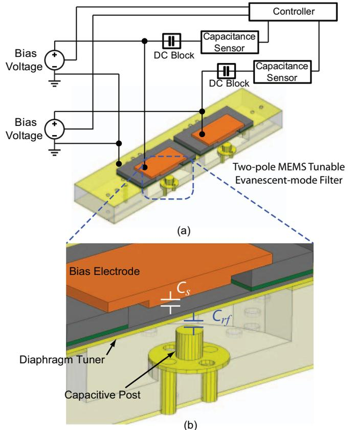
Fig. 1. (a) Concept illustration of tunable filter monitoring through capacitance measurement. (b) The method relies on the one-to-one relationship between  $C_s$  and  $f_0$  (which is determined by  $C_{rf}$ ).
