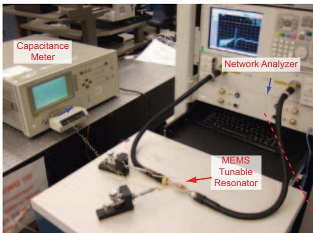
Fig. 6. Picture of the measurement setup.
