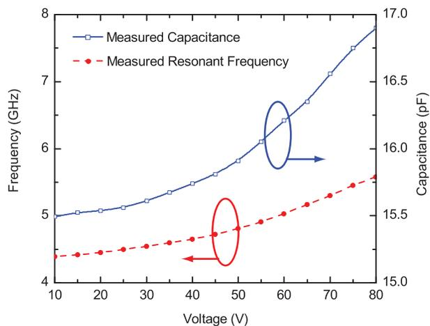
Fig. 7. Measured  $C_s$  and resonant frequency with respect to bias voltage.
