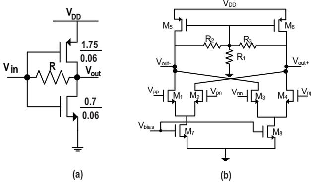
Fig. 3. (a) The unit  $G_m$  cell that is used with different scaling factors (b) The differential difference amplifier
