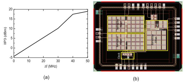
Fig. 10. (a) Simulated out-of-band IIP3 of the filter for different offset frequencies from center frequency of the filter. ( $f_{io}=1$  GHz) (b) Chip layout of the proposed filter.
