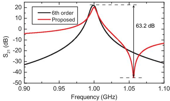
Fig. 5. Comparison between all pole filter and the proposed filter.
