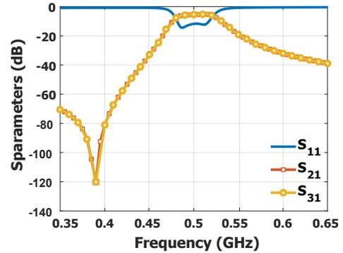
Fig. 3. **Non-modulated** response showing a general 2-pole filter characteristics with a flat passband and two poles in the return loss.
