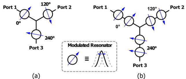
Fig. 1. Magnetic-free circulator based on STM of (a) resonator and (b) 2-pole bandpass filter.
