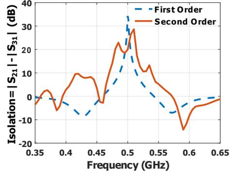
Fig. 6. Simulated isolation performance for circulators with single resonator and 2-pole filters.
