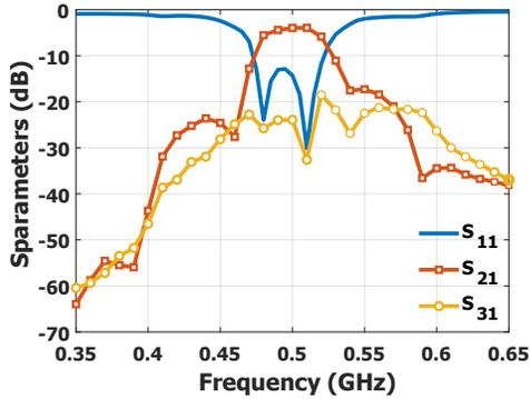
Fig. 4. Simulated S-parameters of the proposed circulator based on STM of 2-pole filters
