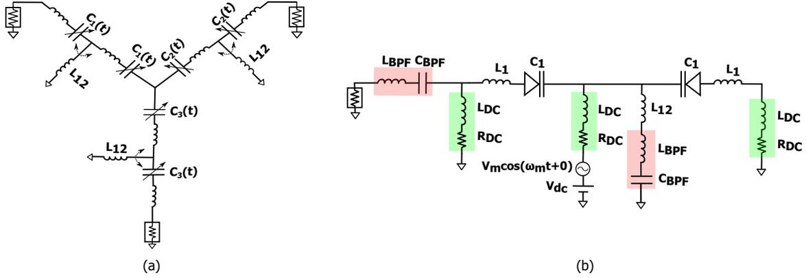
Fig. 2. Proposed circulator architecture: (a) 2-pole bandpass resonators connected in a Y topology and (b) practical implementation of a time-varying capacitor using varactors along with the necessary biasing network and filters.
