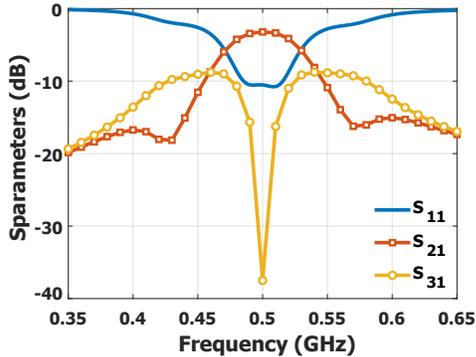
Fig. 5. Simulated S-parameters of the circulator based on STM of single resonators.
