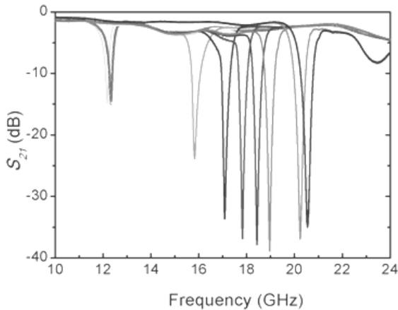
**Figure 6.** Measured  $S_{21}$  results of 12 GHz to 21 GHz tuning 2-pole bandstop filter.
