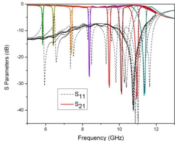
**Figure 7.** Measured results of the 6 GHz to 12 GHz tuning 2-pole filter across the tuning range.
