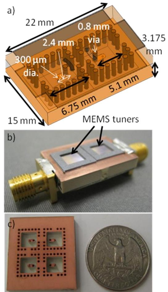
**Figure 5.** 6 GHz to 12 GHz tuning filters. a) Simulation model of 2-pole filter. b) Fabricated 2-pole filter. c) Fabricated 4-pole filter
