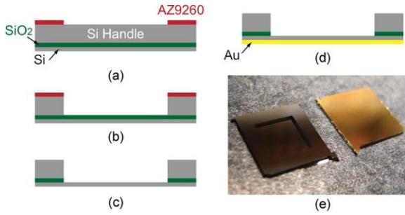
**Figure 2.** Fabrication process for MEMS diaphragm. a) AZ9260 patterning. b) DRIE. c) Oxide etch. d) Au sputter. e) Fabricated MEMS diaphragm.
