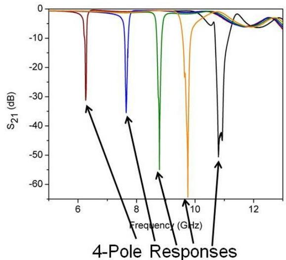
**Figure 8.** Measured results of the 6 GHz to 12 GHz tuning 4-pole filter across the tuning range.
