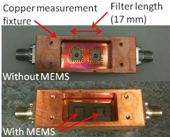
**Figure 4.** Photographs of the 12 GHz to 21 GHz filter with and without MEMS in a measurement fixture.
