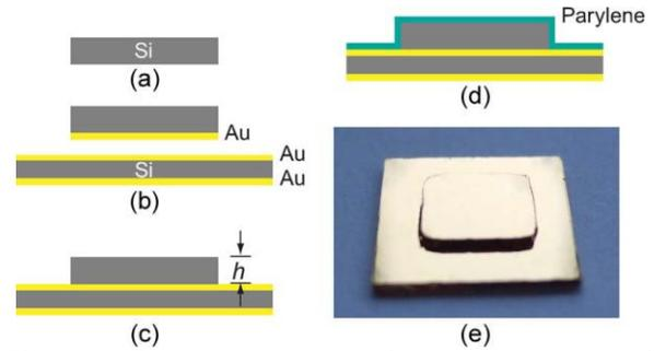
**Figure 3.** Fabrication process for bias electrodes. a) Top silicon piece. b) Au sputter. c) Au-Au thermal compression bonding. d) Parylene deposition. e) Fabricated electrode.
