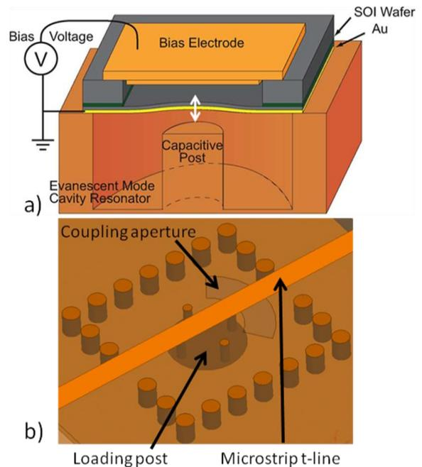
**Figure 1.** a) 3-D model of highly-loaded coaxial cavity with MEMS tuner and bias electrode. b) Substrate-integrated bandstop implementation
