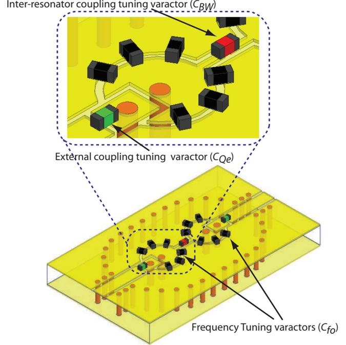
Fig. 1. Proposed substrate-integrated 3-D coaxial cavity two-pole filter and close up of top surface showing the various lumped components
