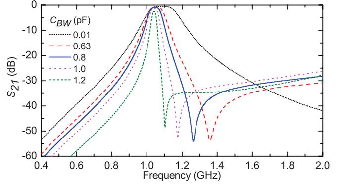
Fig. 3. Ansys HFSS filter simulation shows that as  $C_{BW}$  increases and becomes significant, BW decreases and a transmission zero appears above the passband.
