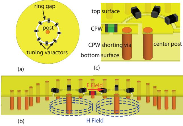
Fig. 2. (a) Previously demonstrated resonator in [5] and [6] and (b) proposed mixed inter-resonator magnetic and electric coupling. (c) Tunable external coupling structure where CPW is shorted from top to bottom surface.
