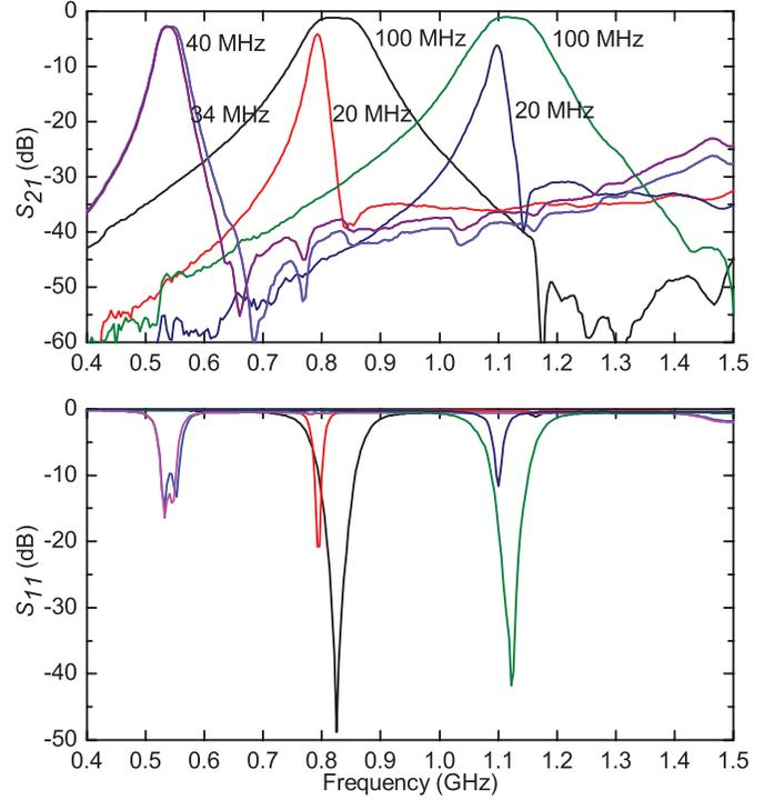
Fig. 6. Measured (a)  $S_{21}$  and (b)  $S_{11}$  showing the maximum and minimum bandwidths at selected frequencies. The filter can continuously tune center frequency and BW.
