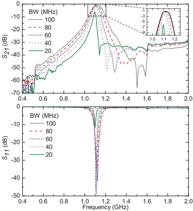
Fig. 5. Measured  $S_{21}$  for fabricated two-pole tunable filter. Both BW and TZ frequency decrease as  $k_E$  is increased.
