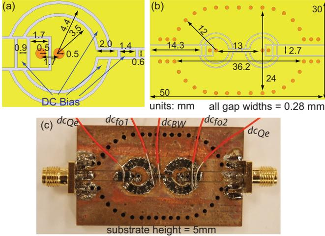
Fig. 4. Designed filter dimensions (units in mm) with (a) close up and (b) full view. (c) Fabricated filter with back-to-back varactors.
