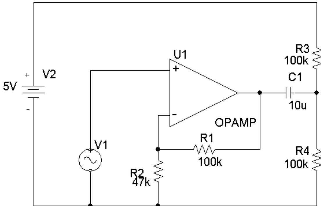
**Figure 4**, triangle wave amplifier
