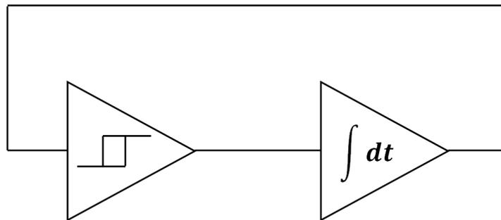
**Figure 1**, block diagram for triangle wave generator
