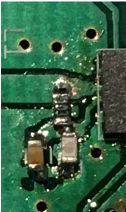
**Figure 7**, RF trace shunt elements
