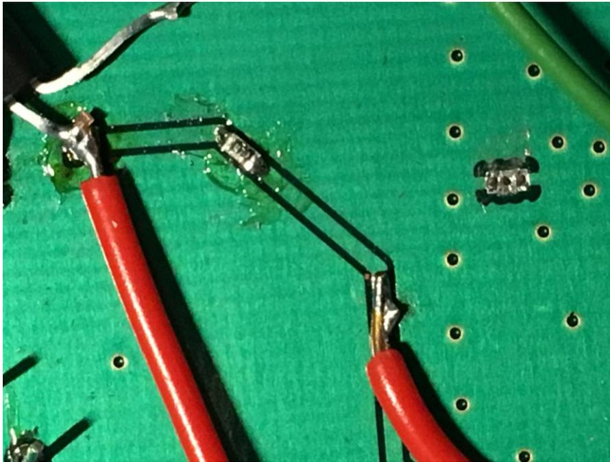
**Figure 5**, improvised SMT pad and fly wire connection
