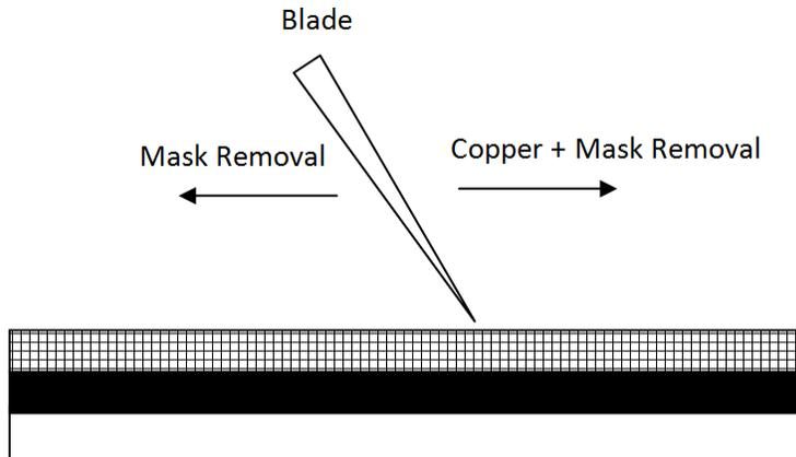
**Figure 6**, Scraping direction for material removal
