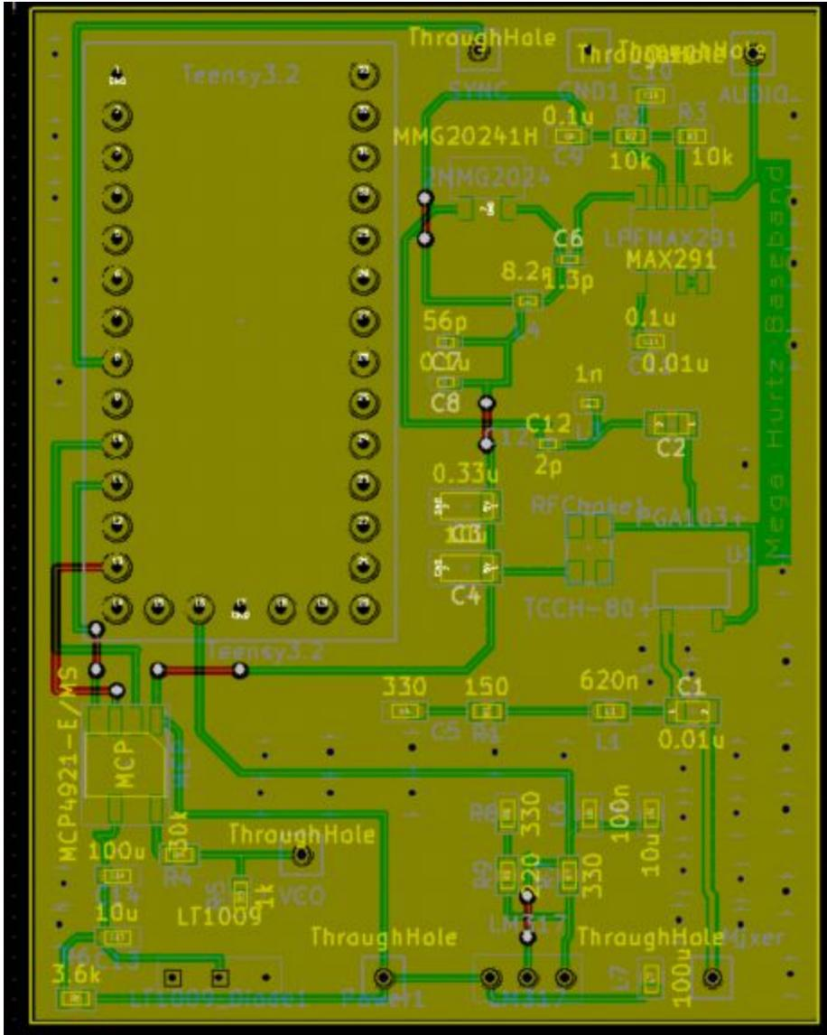
Figure 7. Complete Design of Baseband Board.
