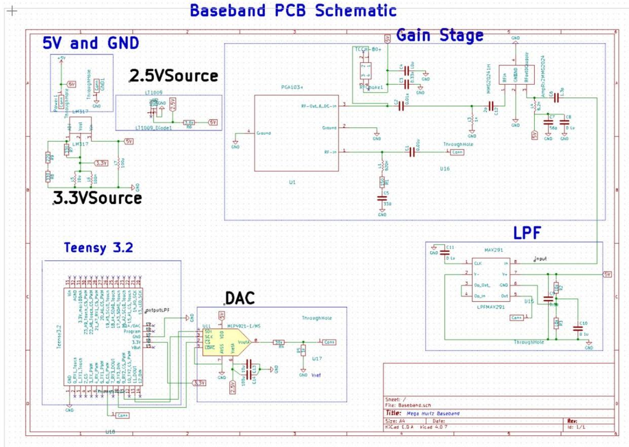
Figure 1. Baseband Schematic
