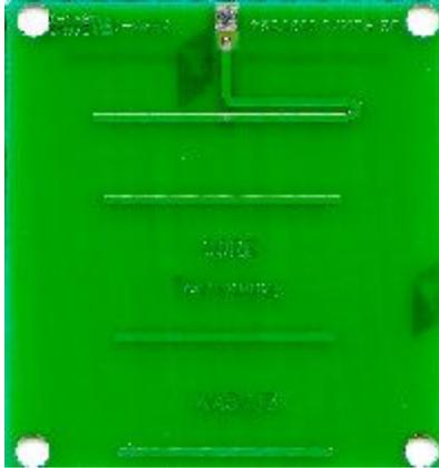
Fig 2. Yagi Antenna
