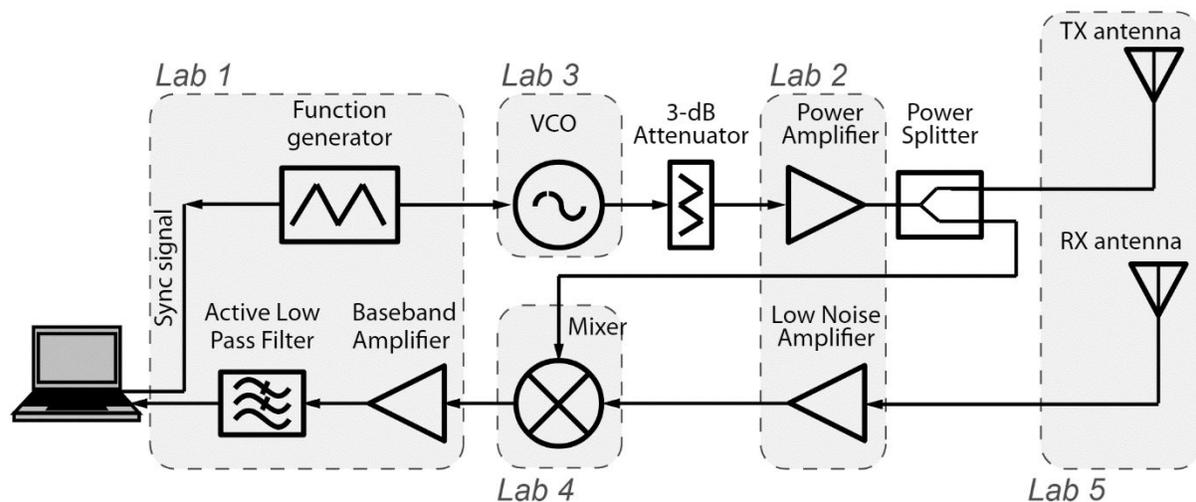
Fig 1. Radar System Design Quarter 1
