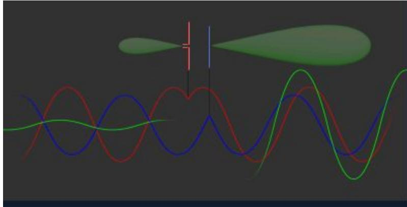
Fig 4. Directionality of a Yagi Antenna
