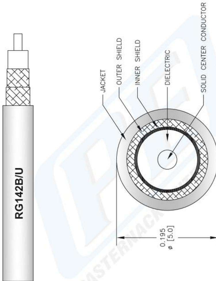
To prepare the RF cable, we need to create exposing cores as shown as the left part of the upper graph at both sides for a certain length of cable. As mentioned above the large diameter of the cable renders most clipping and stripping tools available in our lab useless. Specific RG142 tools are available online but they are expensive thus
