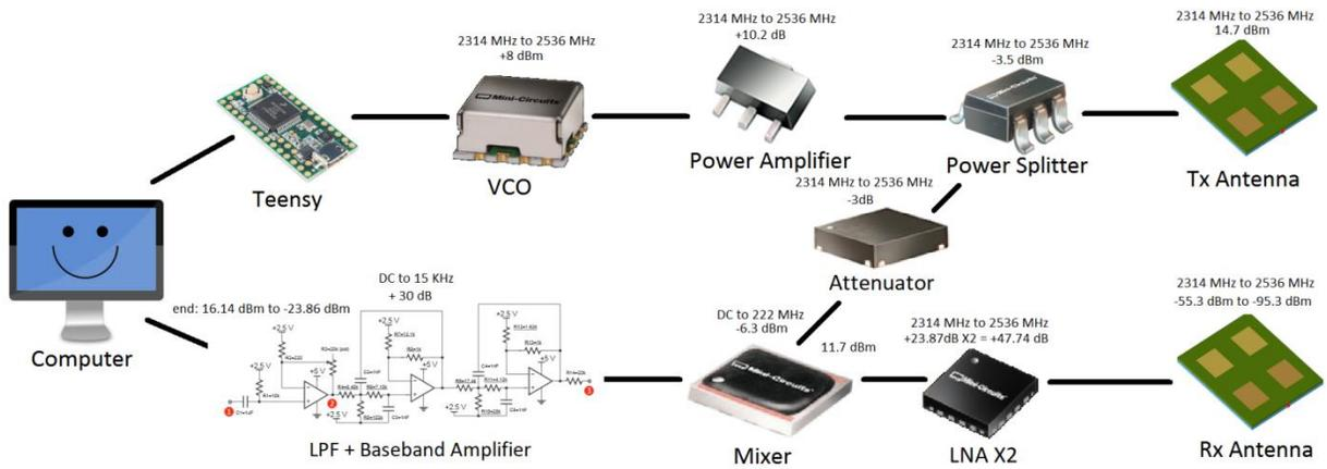
**Fig 4.** Block diagram and component of our FMCW radar system.
