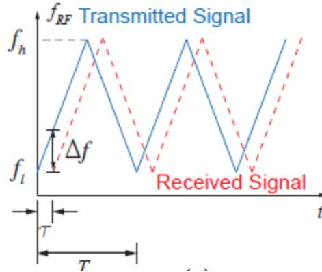
**Fig 2.** Wave form of the transmitted and received signal.
