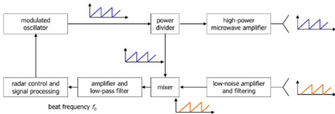
**Fig 1.** The FMCW radar system.
