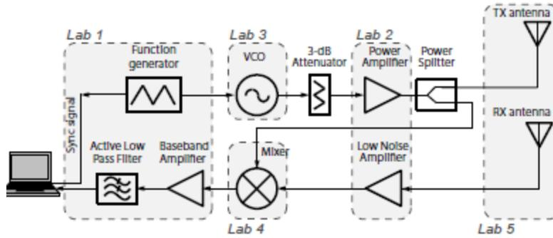
**Fig 3.** Block diagram of the FMCW radar system.
