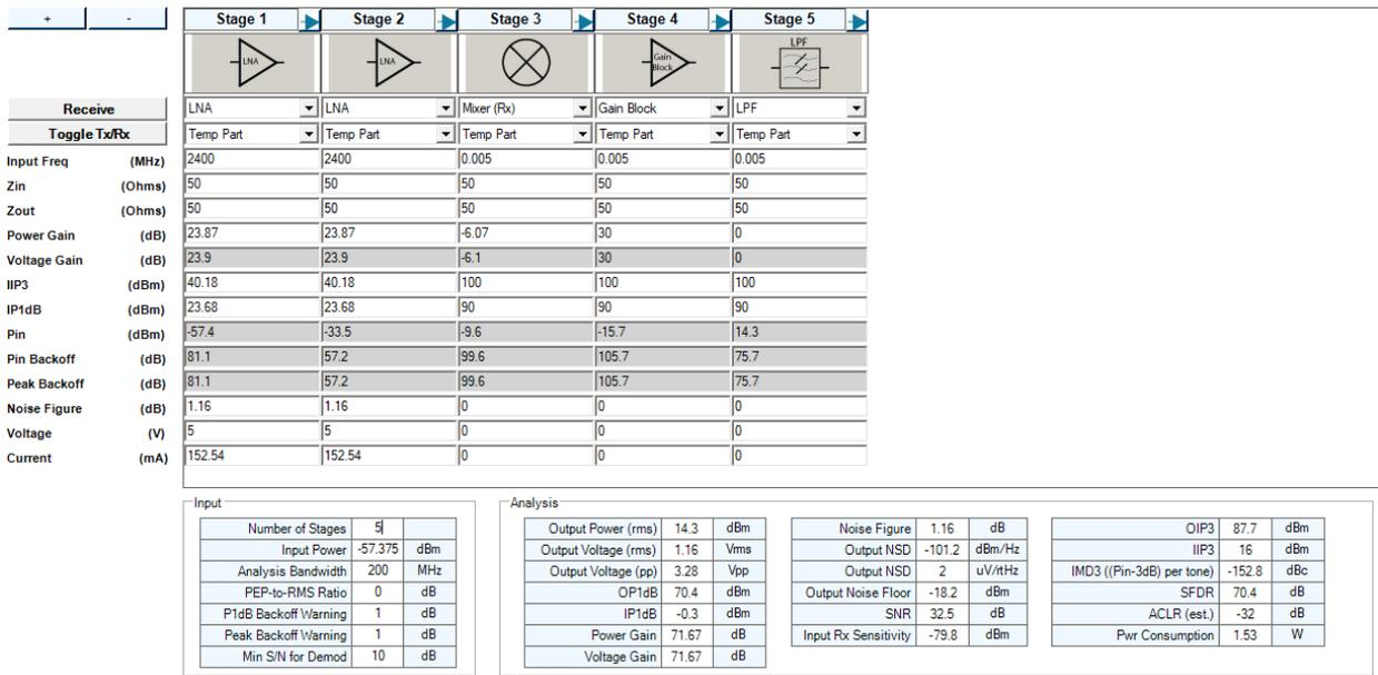
Fig 6. The ADIsimRF simulation of the receiver side.
