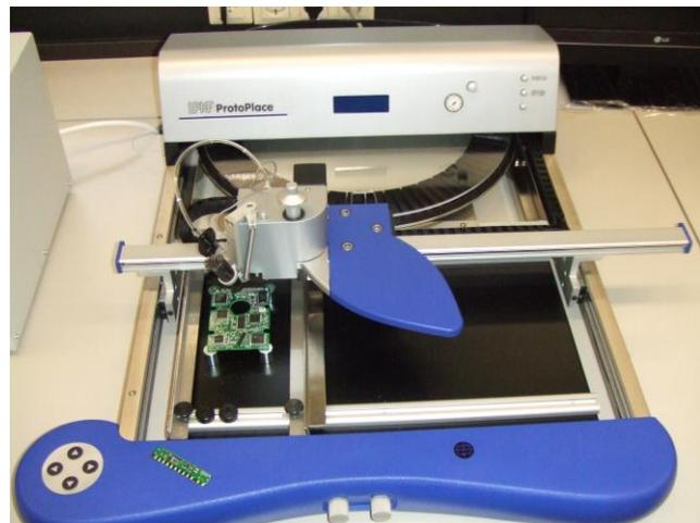
Figure 3. Images of ProtoFlow S and ProtoPlace S
