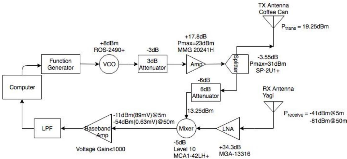
Fig.1 Complete Design Block Diagram
