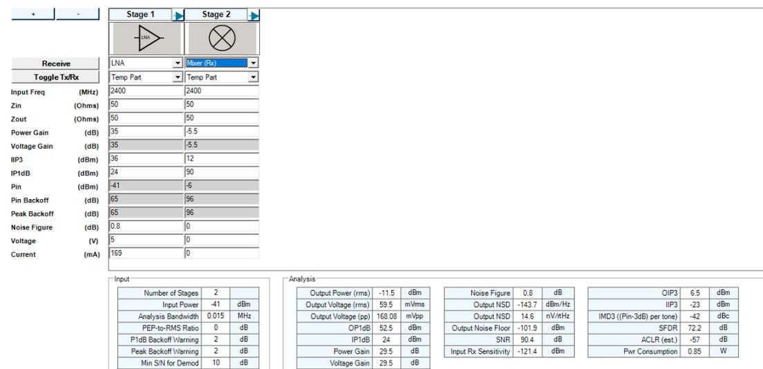
Fig.3 Receiver Simulation
