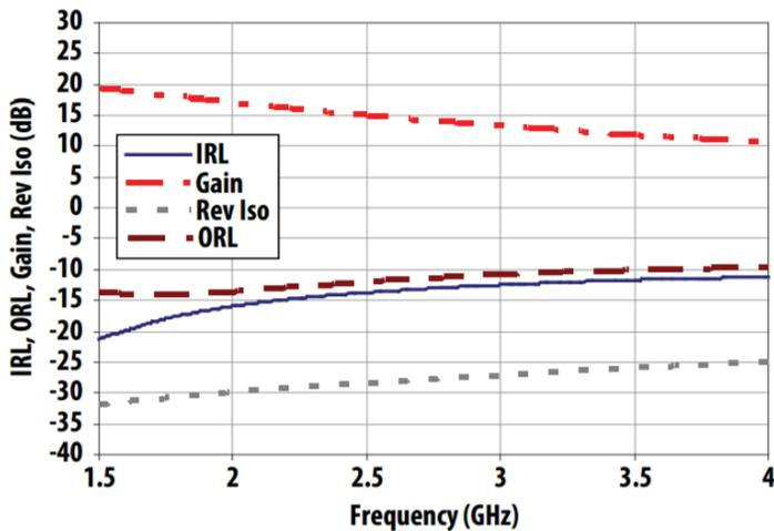
Note: Notice how the gain rapidly diminishes with respect to frequency. If we wanted to operate at a range of 2.3-2.5 GHz, we would observe a 5-6 dB gain drop.
