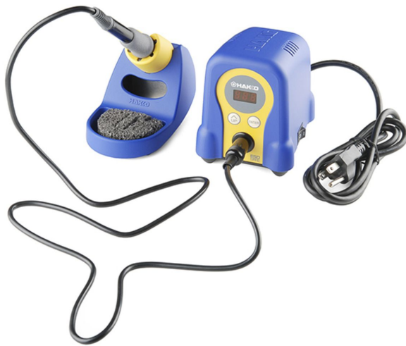
Figure 3-a. Soldering iron station
